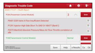
The tested system with fault code appears in red and the system with OK displays in black (normally).
