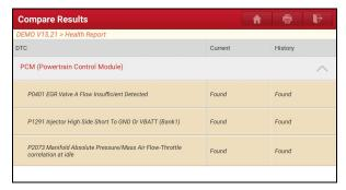
Current indicates DTC status of post-repair.
